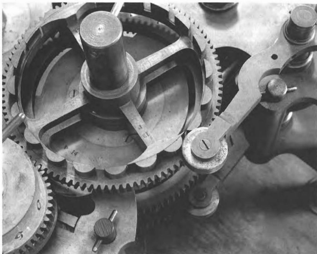
FIGURE 1.3 Difference Engine Cogs details. Demonstration model of Babbage's Difference Engine No. 1, nineteenth century. Credits: Science Museum (London) / Science & Society Picture Library.
